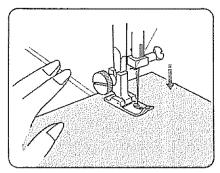
Before sewing with the straight stitch 7. At the end of the seam, you may foot, be sure the stitch selector dial is set to the center needle position.
